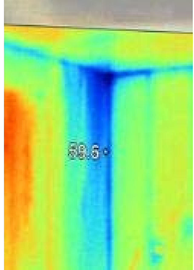
Water Behind the wall that has been captured by the IR camera.
